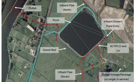
Figure 1 Ngaruawahia WWTP alout, showing headworks (influent screen) location
