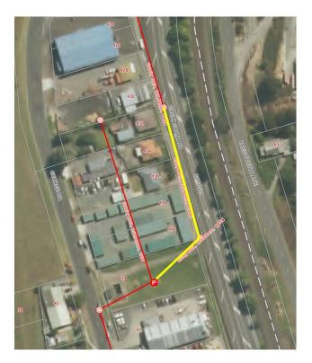
Replacement of old iron pipe with plastic for high pressure waste line from pumping station to connection at the south end of town is ongoing. Yellow section is being replaced.
