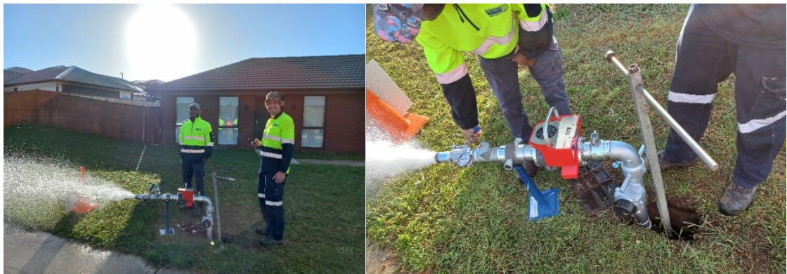
Figures 1 and 2: Staff from Detection Services carrying out hydrant flow testing (with assistance from the Watercare Project Manager).
