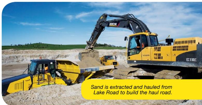
Sand is extracted and hauled from Lake Road to build the haul road.
