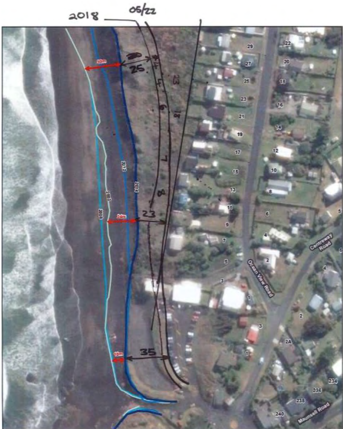
Figure 2: Erosion at Sunset Beach
