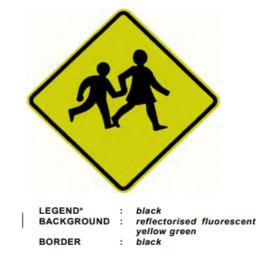
The symbol shall be oriented such that the pedestrians appear to be walking towards the roadway; eg where the sign is installed on the right hand side of the road, the symbol must be reversed.
