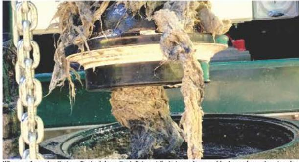
Wipes and nappies that are flushed down the toilet contribute towards many blockages in wastewater pipes.
