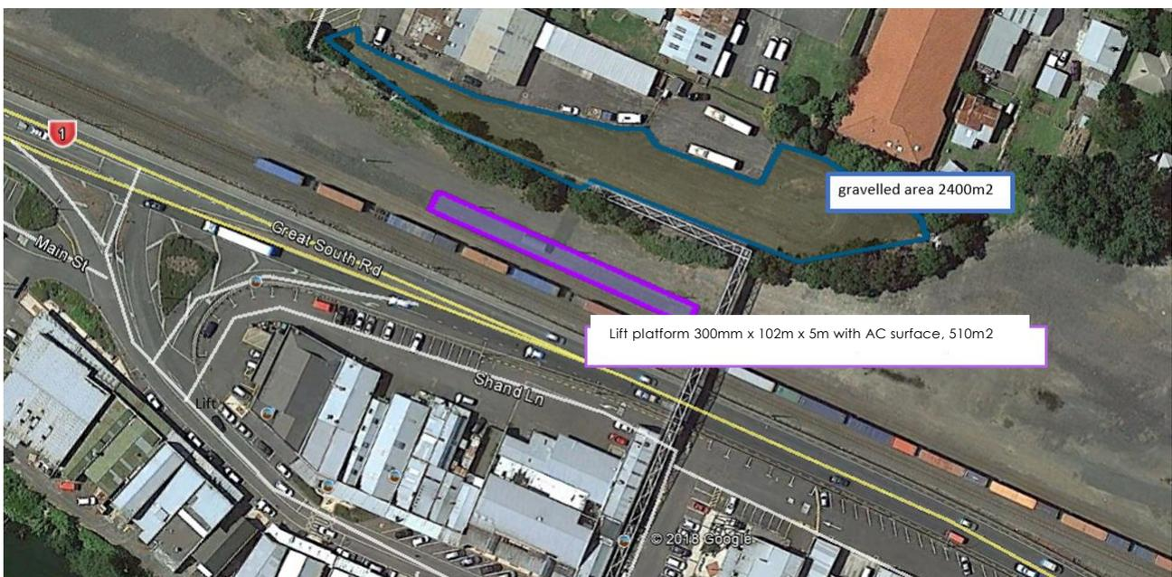
Figure 10-3: Concept layout for Huntly Station
