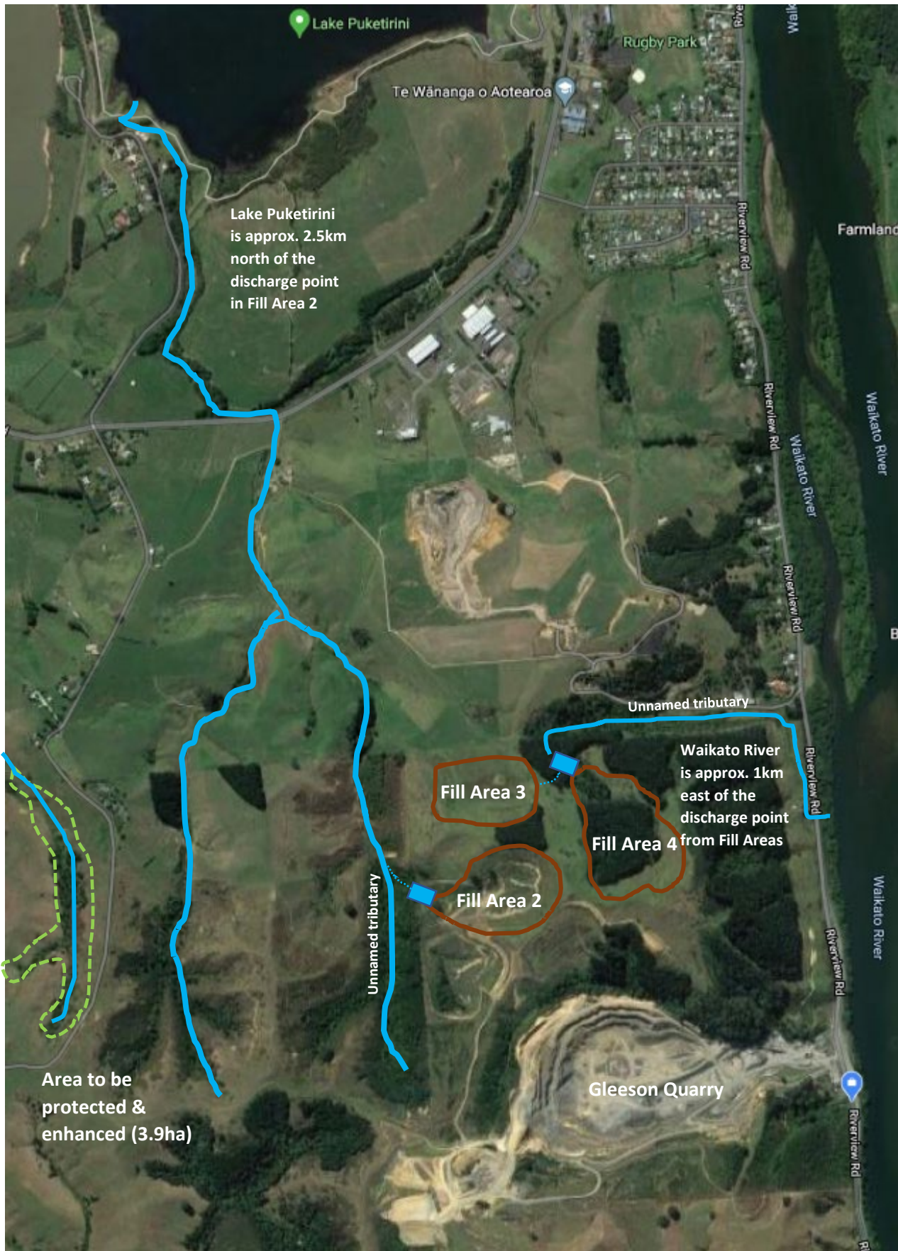
Any clean water discharge from Fill Area 2 flows 2.5km before discharging into Lake Puketirini. Clean water discharge from Fill Areas 3 and 4 flows 1km before discharging into the Waikato River
