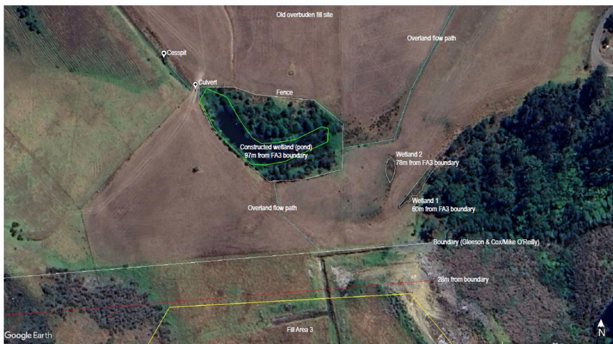
Figure 1: Aerial Plan depicting location of artificial and induced wetlands – note the 60m (Wetland 1) measurement includes the 28m measurement shown on Gleeson land, as this is the closest the managed fill activity can be to the boundary (geotechnical requirement). The discharge point will be closer to the boundary (approximately 35m) as discussed in this memo.
