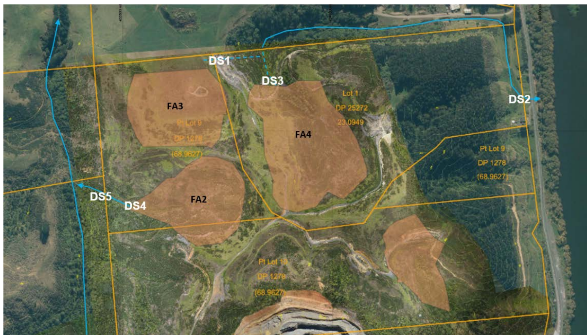
Figure B-1 Fill Areas: Storm Water Clarity Sampling Points
