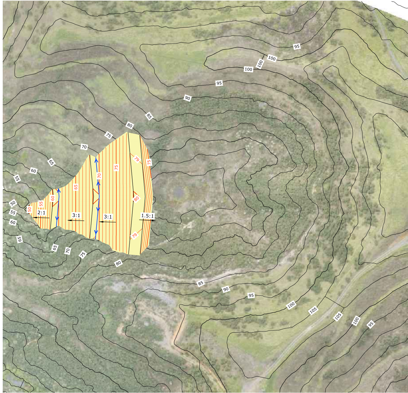
STAGE 2.2: STRUCTURAL FILL (BUND) LAYOUT SCALE 1:2000
