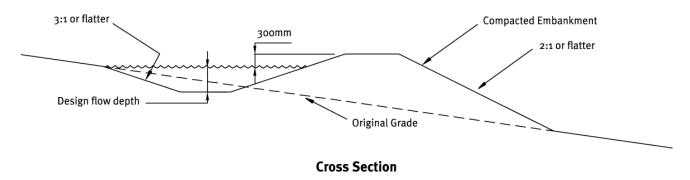
Figure 3: Cross-section of a dirty water diversion.
