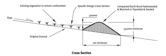
Figure 2: Cross-section of a clean water diversion bund.
