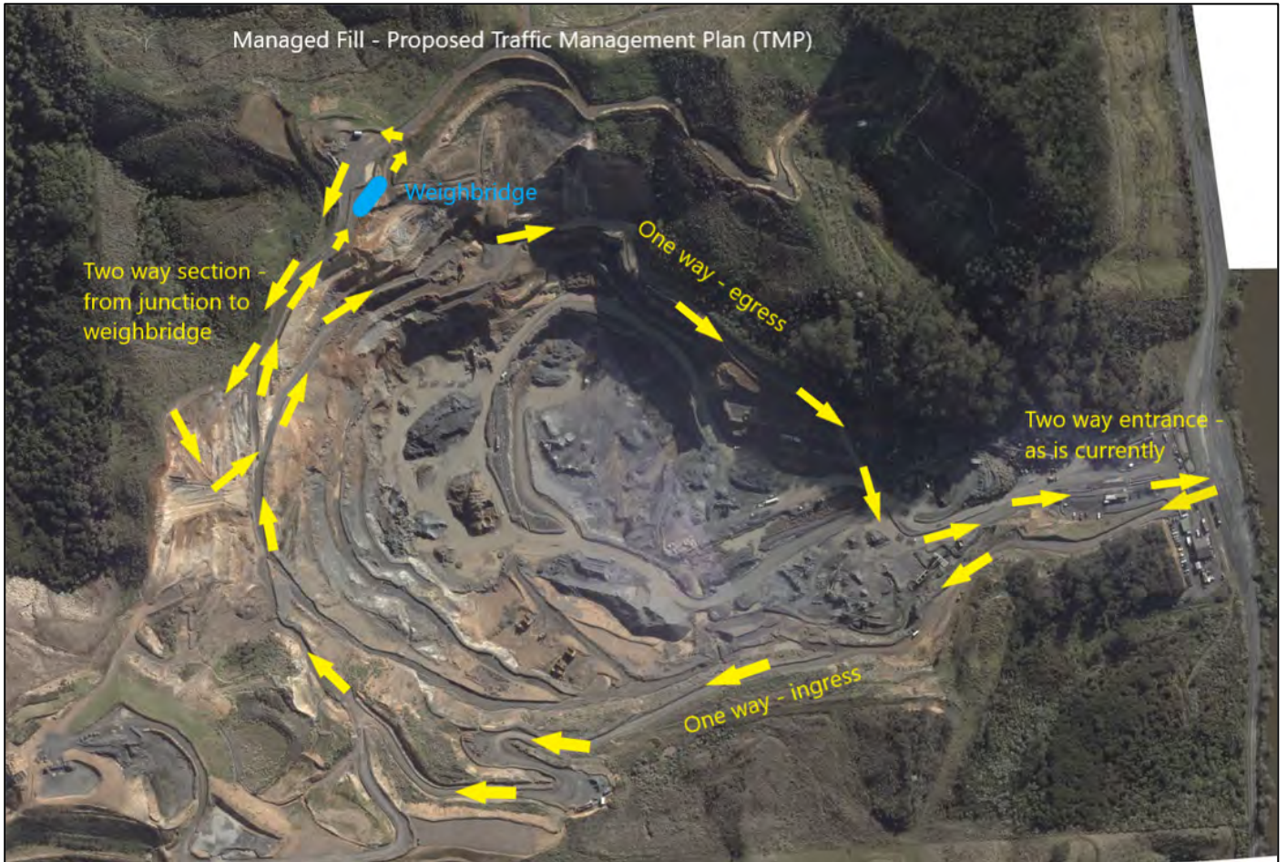
Figure 3: Proposed Traffic Management Plan shows internal one way arrangement and the proposed additional weighbridge located inside the site.
