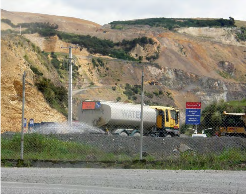
Water being applied as dust suppressant in Oct 2020
