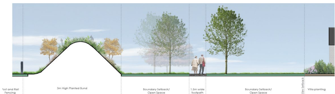
Figure 3: Typical Boundary Treatment to western boundary. Features 25m built form setback, open space and planting and 3m high planted bund. Refer BML Landscape Concept Package.
