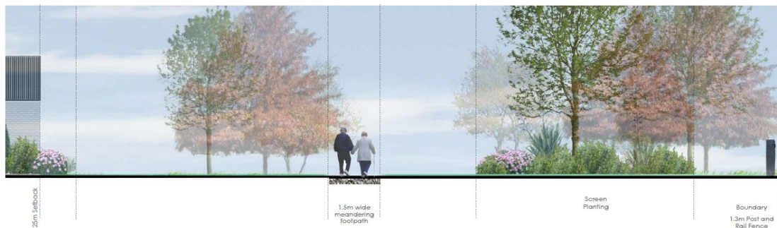
Figure 2: Typical Boundary Treatment to southern and western boundary. Features 25m built form setback and screen planting. Refer BML Landscape Concept Package.
