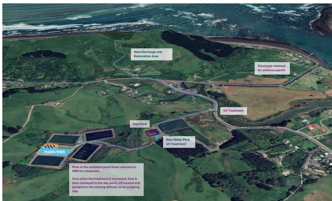
Figure 2-3. Location of the proposed MABR/MBR, pump station and UV treatment, and outfall location.
