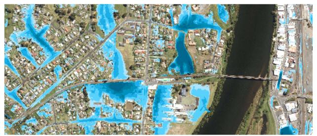
Figure 3: Blockage Scenario 2 – Shows a slight increase in flooding from the base model and a reduction in flood level from the 100% blockage scenario as would be expected. Result: Not considered a critical factor in the flood model as very similar to base model.
