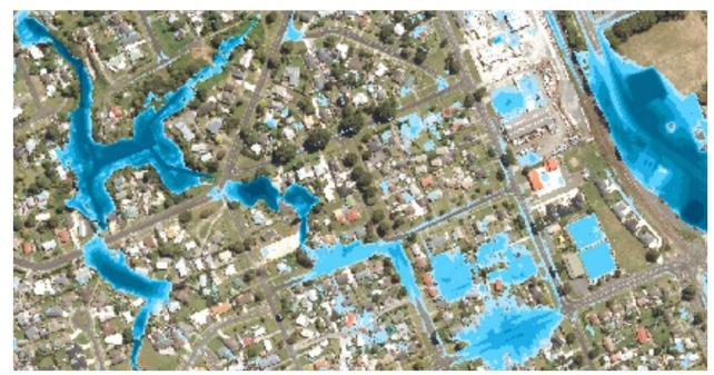
Figure 3: Blockage Scenario 2 – Shows a slight increase in flooding from the base model and a reduction in flood level from the 100% blockage scenario as would be expected. Result: Not considered a critical factor in the flood model as very similar to base model.
