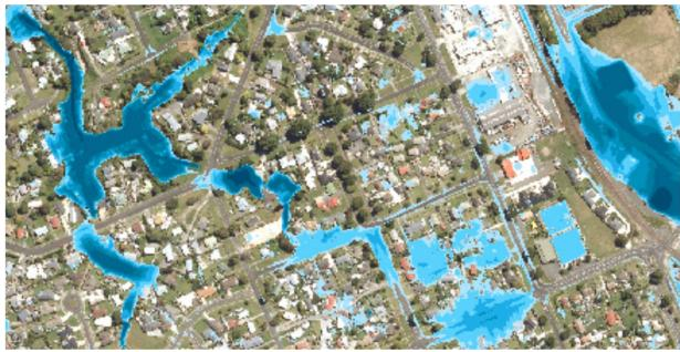
Figure 2: Blockage Scenario 1 – Shows increased flooding by the 100% blockage scenario. This shows an increase in flood levels but still contain within the gully areas. This blockage scenario is unlikely to occur as large culverts are less likely to completely block. No difference in areas that are not constrained by culverts. Result: Not considered a critical factor.
