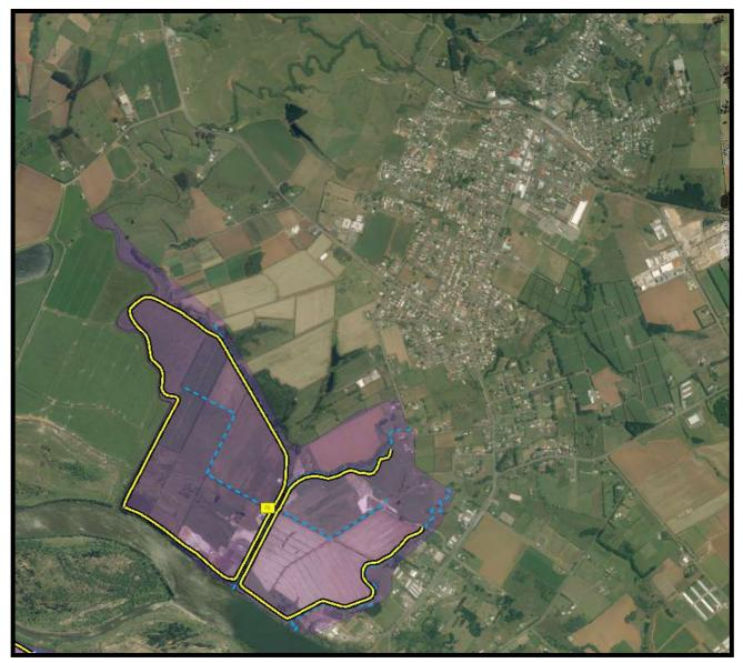
Figure 3 WRC's Tuakau Swamp Drainage Scheme also showing stopbanks and pump station.
