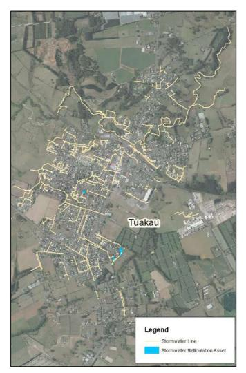
Figure 6 Tuakau existing stormwater system (includes some streams) as provided by WDC GIS data.
