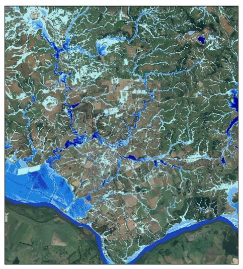
Figure 9 100 year ARI with climate change, rain-on-grid modelling (with first 50mm removed from the results).
