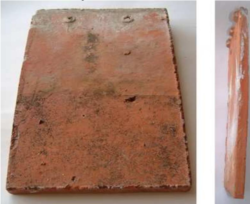
**Sample of the clay tiles used on the factory roof note that only about a third of each tile is ever actually exposed.**
