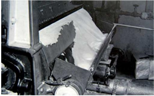
Roller style milk dryer in operation. The milk was sprayed onto the hot surface and then scraped off as the steam heated cylinder rotated.
