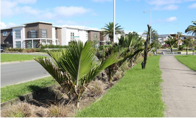
Figure 17. Precedent Image: Swales along the street edge contribute to movement networks, low impact stormwater design and amenity.
