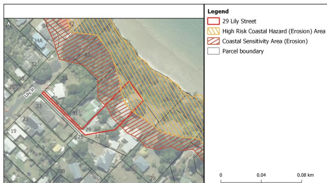
Figure 5: Recommended Coastal Sensitivity Area (Erosion) and High Risk Coastal Hazard Area (Erosion) extents
