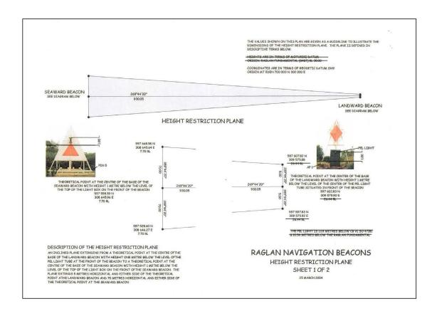
Note: The height of the landward beacon is not fixed in the plan and reference is made to its actual height, whatever that may be at a point in time
