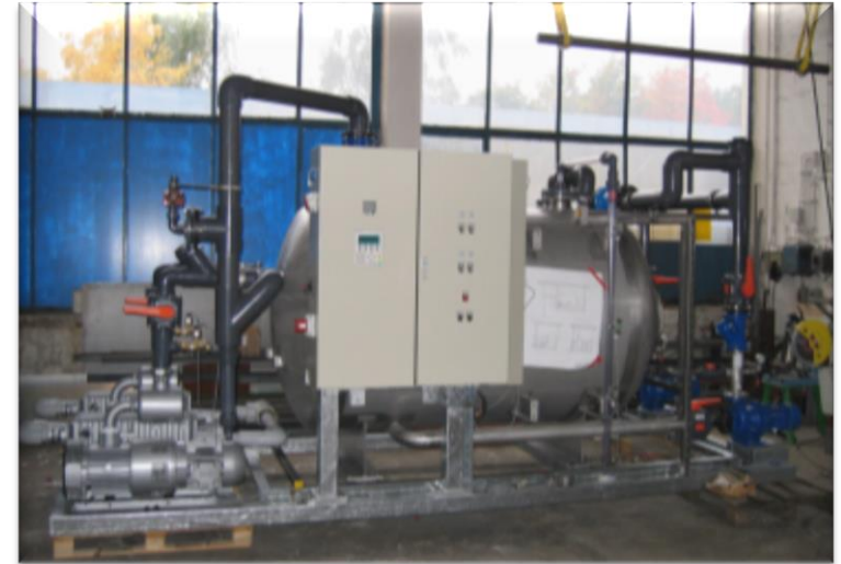
Pre-tested skid mounted pump station in Croatia
