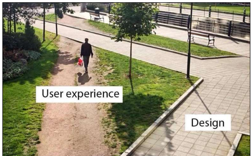
Figure 8: Design route for pedestrians compared with desire line route (User experience) for pedestrians 39
