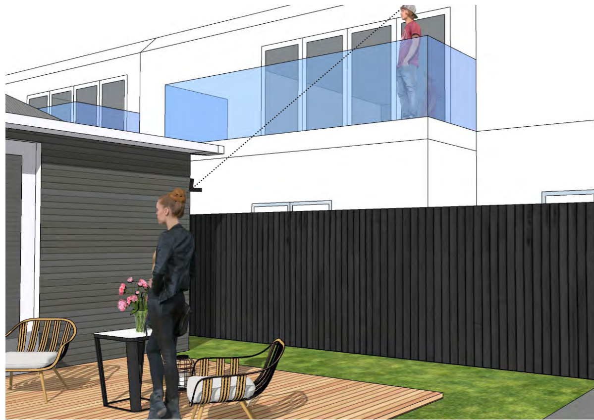
DIAGRAM A2.1: With no controls on the placement of balconies and first floor windows the privacy of the adjoining property is compromised
