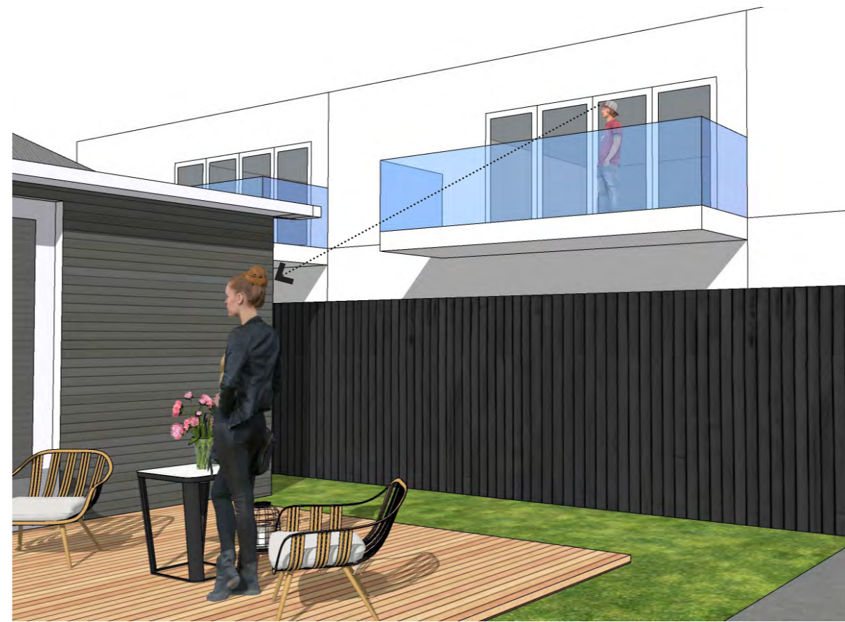
DIAGRAM A2.2: By controlling the placement of balconies and first floor windows within 4m of the boundary it is possible to provide sufficient space to improve privacy outcomes.
