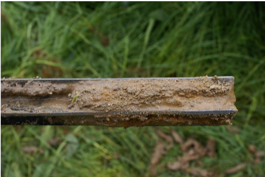
Plate 2: Fully saturated sand near the water table: test site 5
