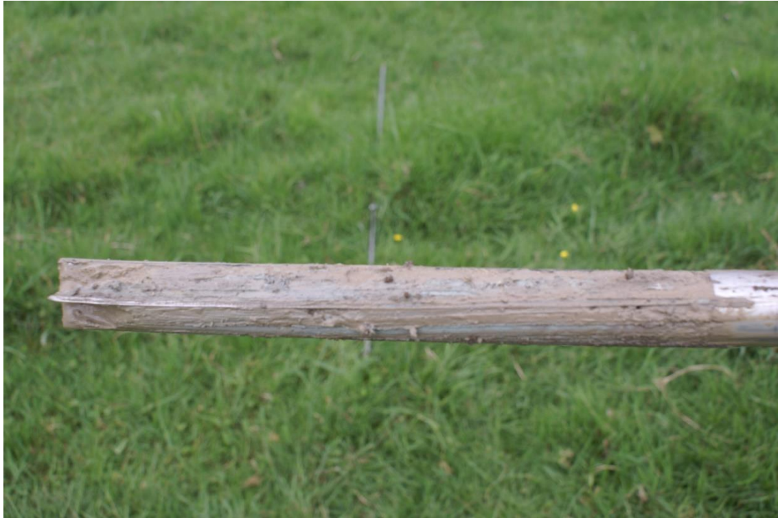
Plate 3: Very soft saturated clay at 1.6 m: Test site 10
