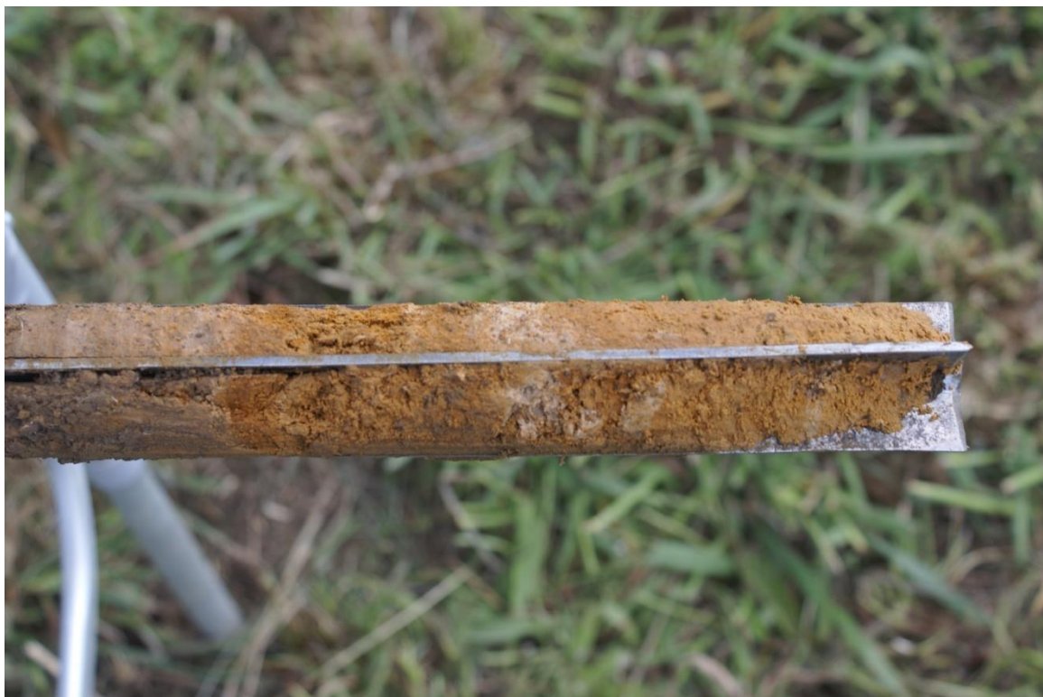
Plate 4: The boundary between grey-brown unit 2 and orange-brown unit 3
