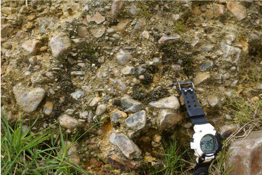
Plate 5: Mixed cobbles, gravel and sand near Site 2
