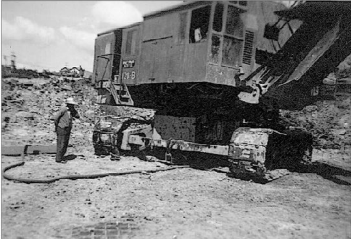
The 120-B electric excavator being viewed by Alexander MacDonald, father of one of the operators Harry MacDonald. During all operations around the machine care had to be taken that the very high voltage cable feeding the several motors were protected. During the repositioning of the 120-B the cable was hefted by hand. An interruption to the power flow would render the machine useless. At one point a second 120-B was added to the mine to increase the removal of overburden. The operating noise within the cab as the various motors spun up and down affected the operators hearing over a period of time. It was not a usual practice for ear-muffs to be worn. The cab had to be rotated so that the steps were above the tracks before access and exit of the operator. A large tonnage of weights were placed at the back of the cab to counterbalance the action of the bucket on the front arm.
