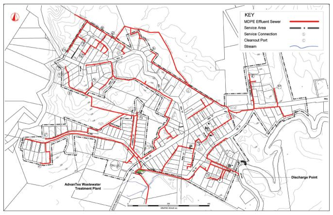
All 198 homes and businesses in Piopio are connected to the Orenco<sup>®</sup> Effluent Sewer and AdvanTex<sup>®</sup> Treatment System. The system has completely eliminated the bad odors that previously emanated from the creek that runs through town.
