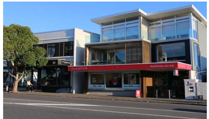
Figure 4. Precedent Image: Steeping back the third storey of the building can assist to maintain a human scale when viewed from the street, and remain in keeping with adjoining buildings.
