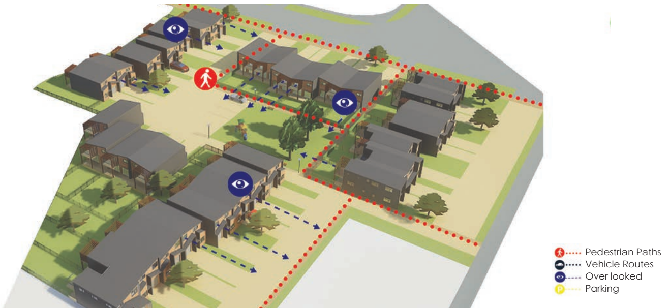
Figure 2. Design pedestrian access ways in a manner consistent with 'Crime Prevention through environmental Design' (CPTED) principles, facilitating passive surveillance; provide dedicated pedestrian access to dwellings and areas of communal open space.
