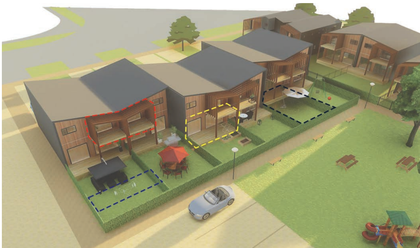
Figure 11. Dwelling layouts designed with a strong indoor-outdoor relationship at ground level (and above - through provision of balconies), garden areas private and well oriented for solar access.
