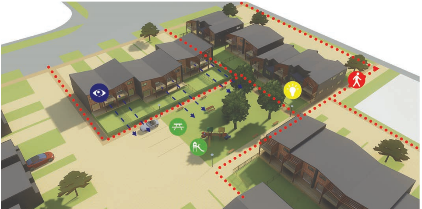
Figure 13. Communal open space overlooked by surrounding dwellings, connected by a dedicated pedestrian network and providing for a range of recreational activities.
