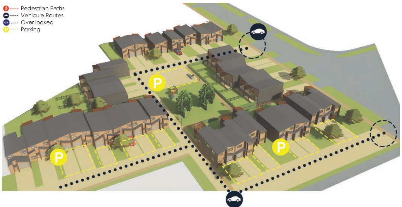
Figure 3. Design an internal movement network that provides for safe circulation and dedicated vehicle access to each dwelling.
