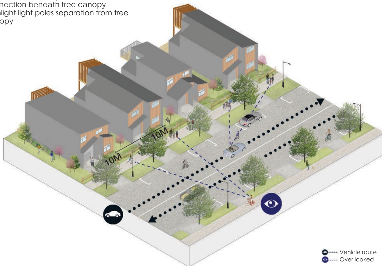
Figure 14. Avoid low shrubs or low canopy trees that block sightlines of pedestrians and vehicles; Generally provide street trees at 10 metre centres, or at an equivalent rate of one tree per residential property, located to avoid interference with services, light poles, driveways and parking bays.
