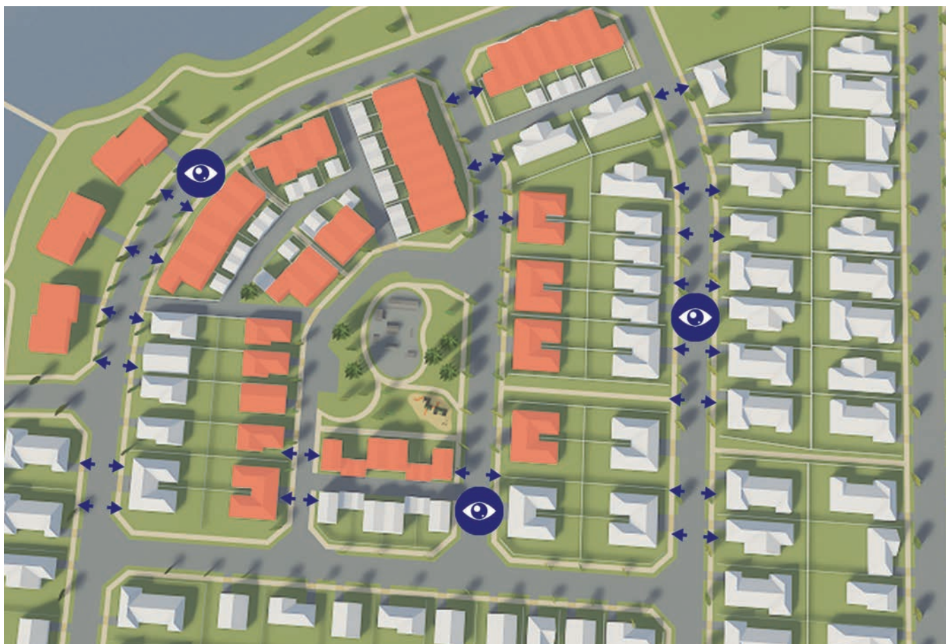
Figure 10. Establish a block layout that enables house fronts on each side of the street to face one another, and place higher density housing adjacent to other features, e.g. public open space
