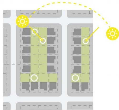
Figure 9. Provide east or west facing open space for streets orientated north-south
