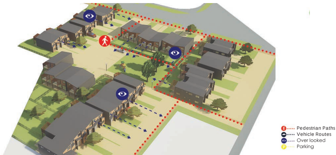
Figure 2. Design pedestrian access ways in a manner consistent with 'Crime Prevention through environmental Design' (CPTED) principles, facilitating passive surveillance; provide dedicated pedestrian access to dwellings and areas of communal open space.
