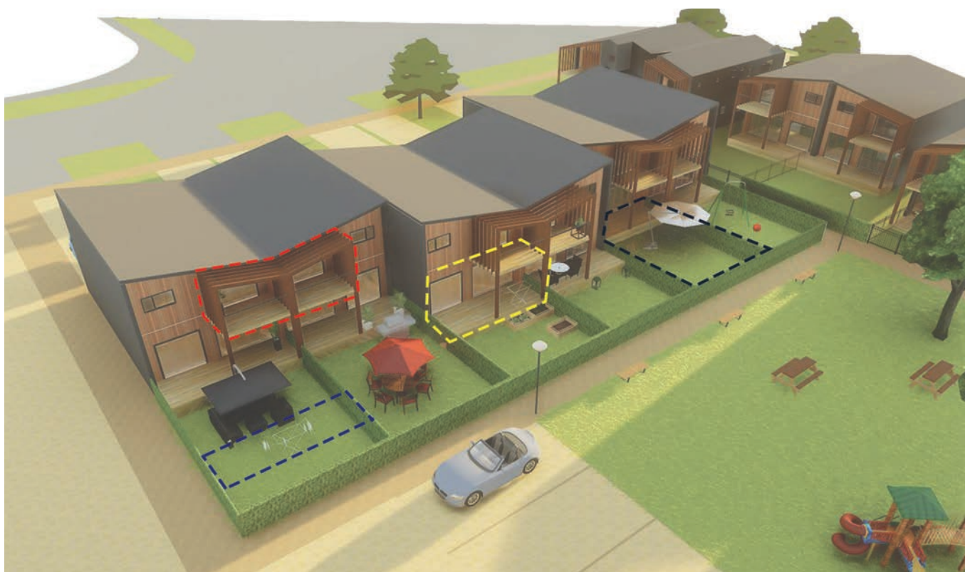
Figure 11. Dwelling layouts designed with a strong indoor-outdoor relationship at ground level (and above - through provision of balconies), garden areas private and well oriented for solar access.
