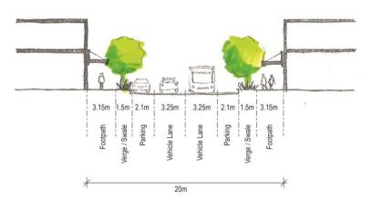
Figure 17. Tuakau Town Centre typical road cross sections: George Street, showing two storey high built form along road corridor
