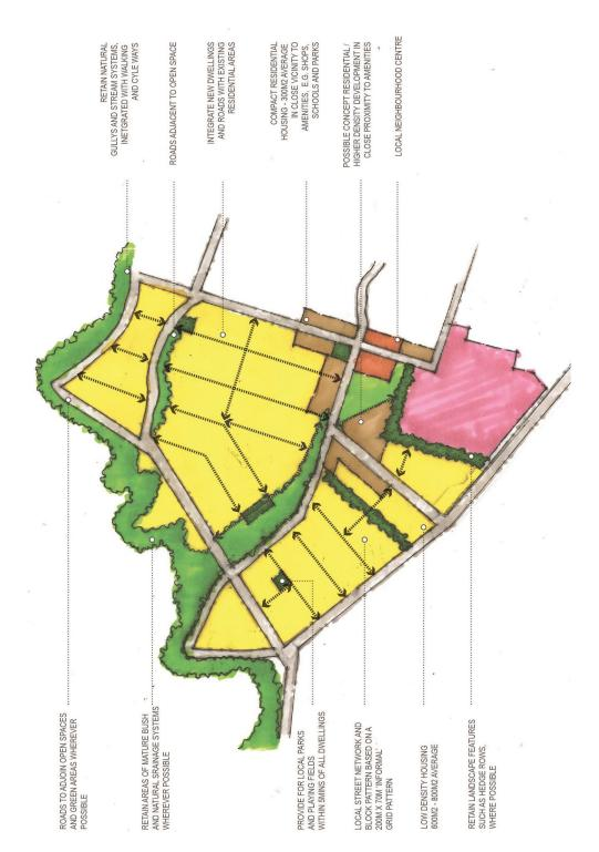
Figure 1. Indicative Development Plan for Taukau's northwestern growth area (Stage 1) illustrating key design principles and outcomes (note, layout is indicative only and subject to future planning and design).
