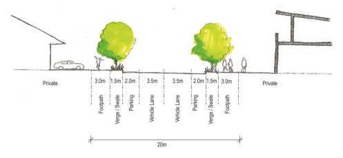
Figure 3. Growth Areas - typical road cross sections: Collector Roads
