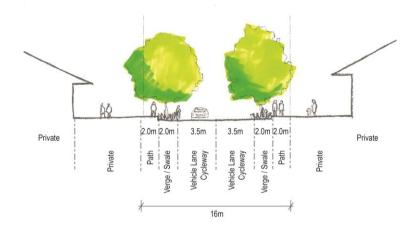
Figure 4. Growth Areas – typical road cross sections: Local Roads (minimising road corridor width where possible)
