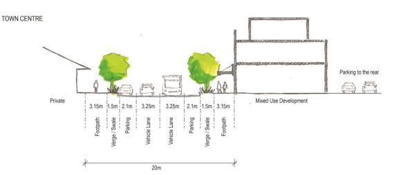
Figure 18. Tuakau Town Centre typical road cross sections: West Street, showing three storey mixed use to east and parking to rear
