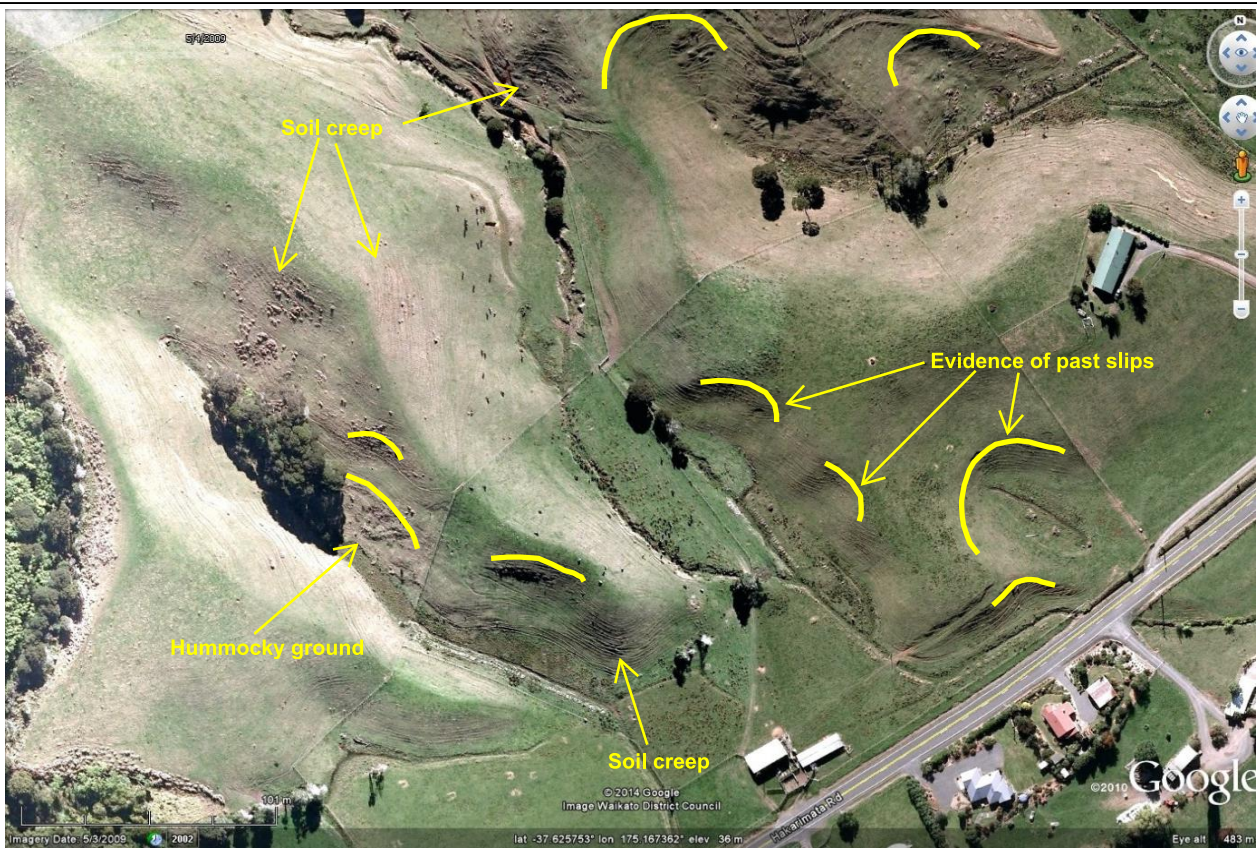
1. This image was taken in May 2009. It shows multiple slips have occurred in the past. Associated with these slips are evidence of hummocky grounds and soil creep.
