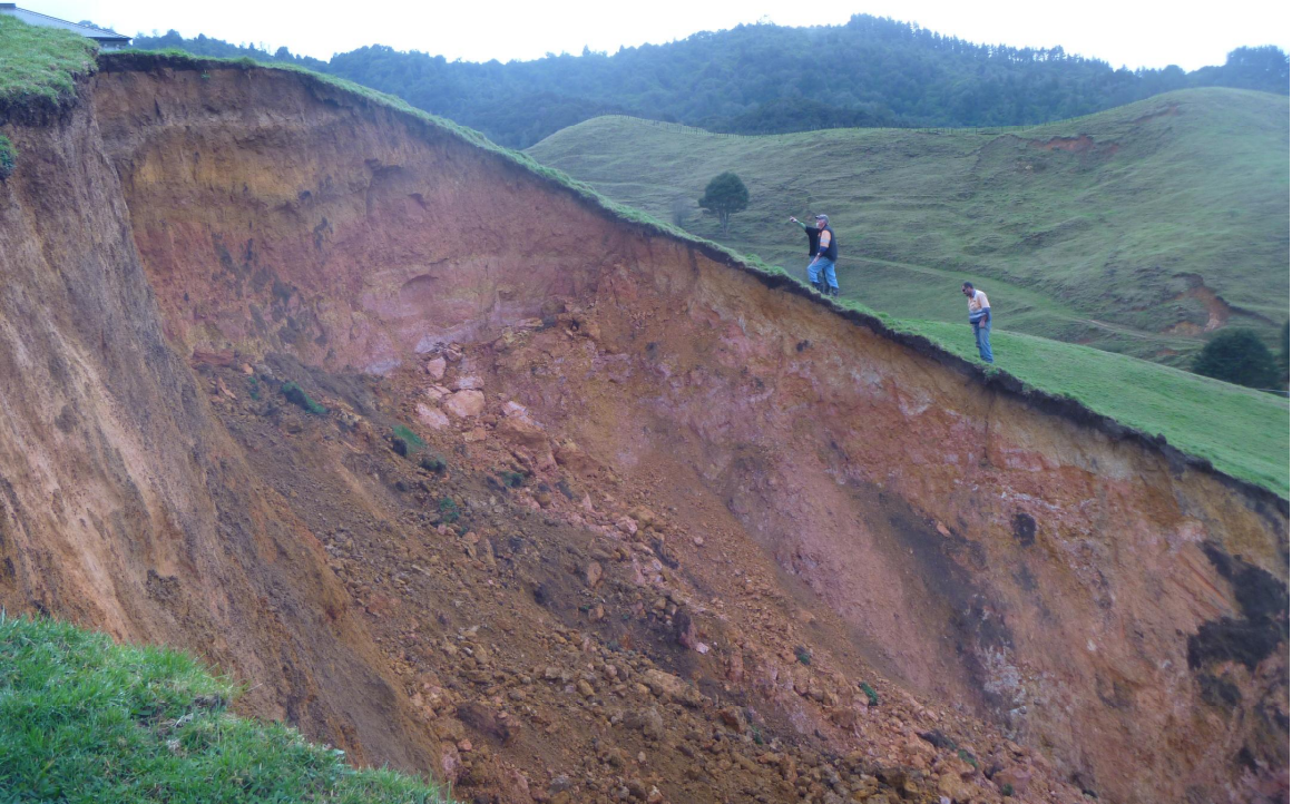
7. The size and depth of back scarp is apparent in this photo
