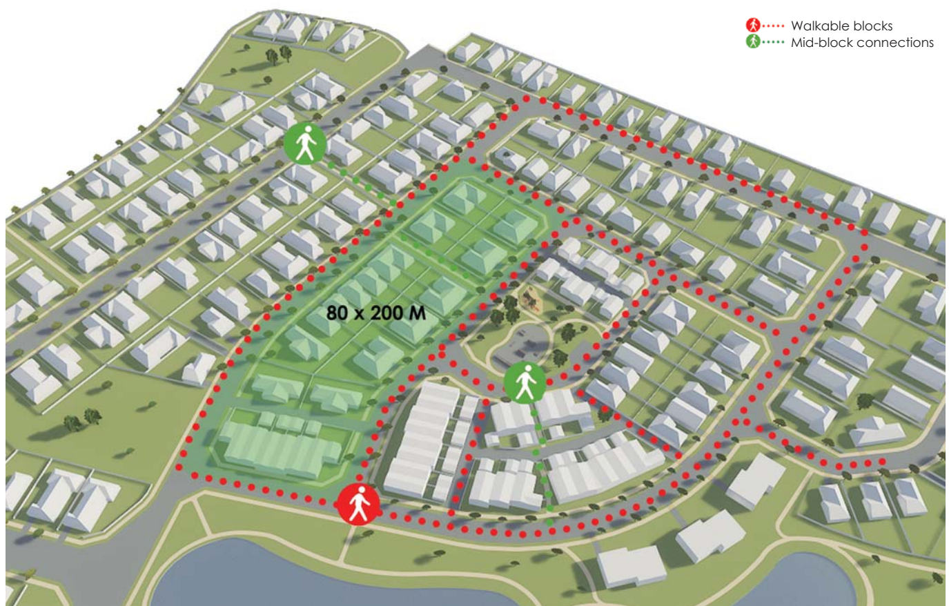
Figure 2. Establish walkable blocks, based on a formal or informal grid; where appropriate, provide short mid-block connections / green links, overlooked by adjoining development.
