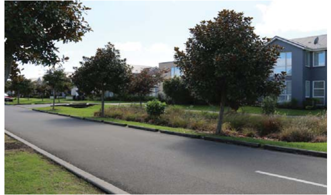
Figure 18. Precedent Image: Swales along the street edge contribute to movement networks, low impact stormwater design and amenity.
