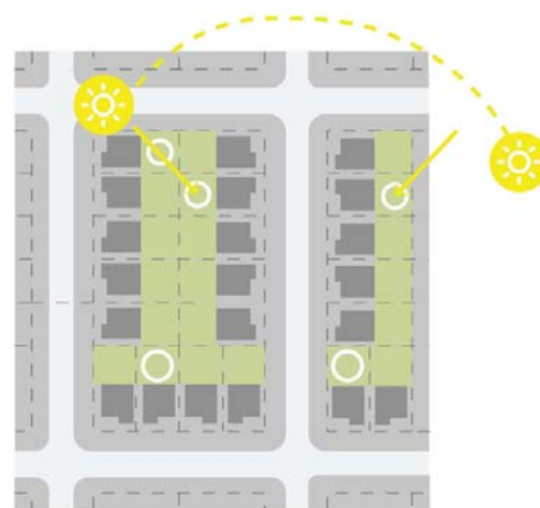
Figure 9. Provide east or west facing open space for streets orientated north-south
