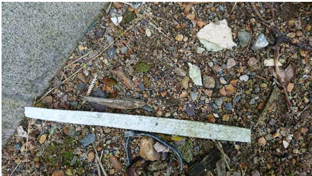
PLATE 4: DAMAGED AND DETERIORATED SUSPECTED ASBESTOS CONTAINING MATERIAL (ACM) AT LOT 1 MILKING SHED
