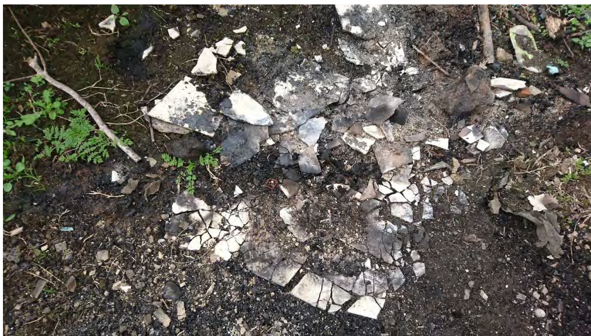
PLATE 12: DAMAGED AND DETERIORATED SUSPECTED ACM FRAGMENTS IN BURN PILE AT LOT 1 MILKING SHED
