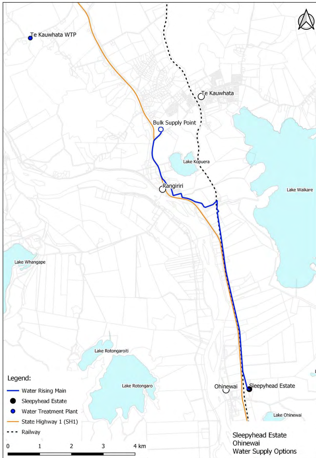
Figure 7: Te Kauwhata Water Treatment Plant Bulk Reticulation Supply Proposed Route
