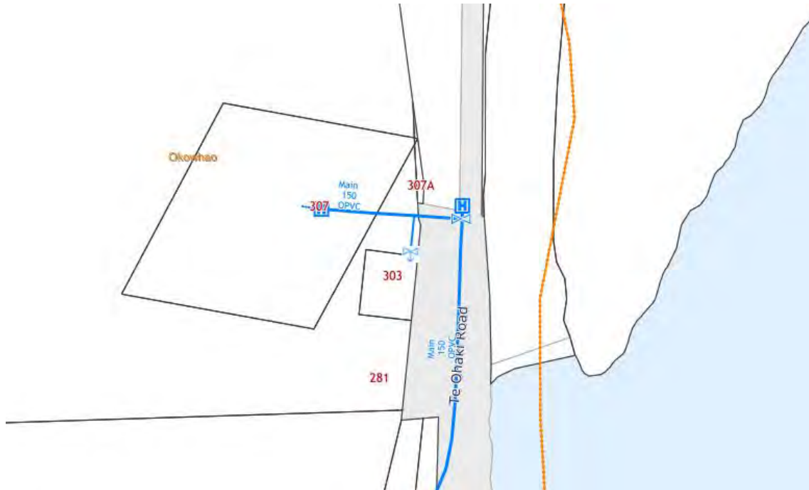
Figure 4: Termination of 150mm dia Supply (source: WDC Maps)
