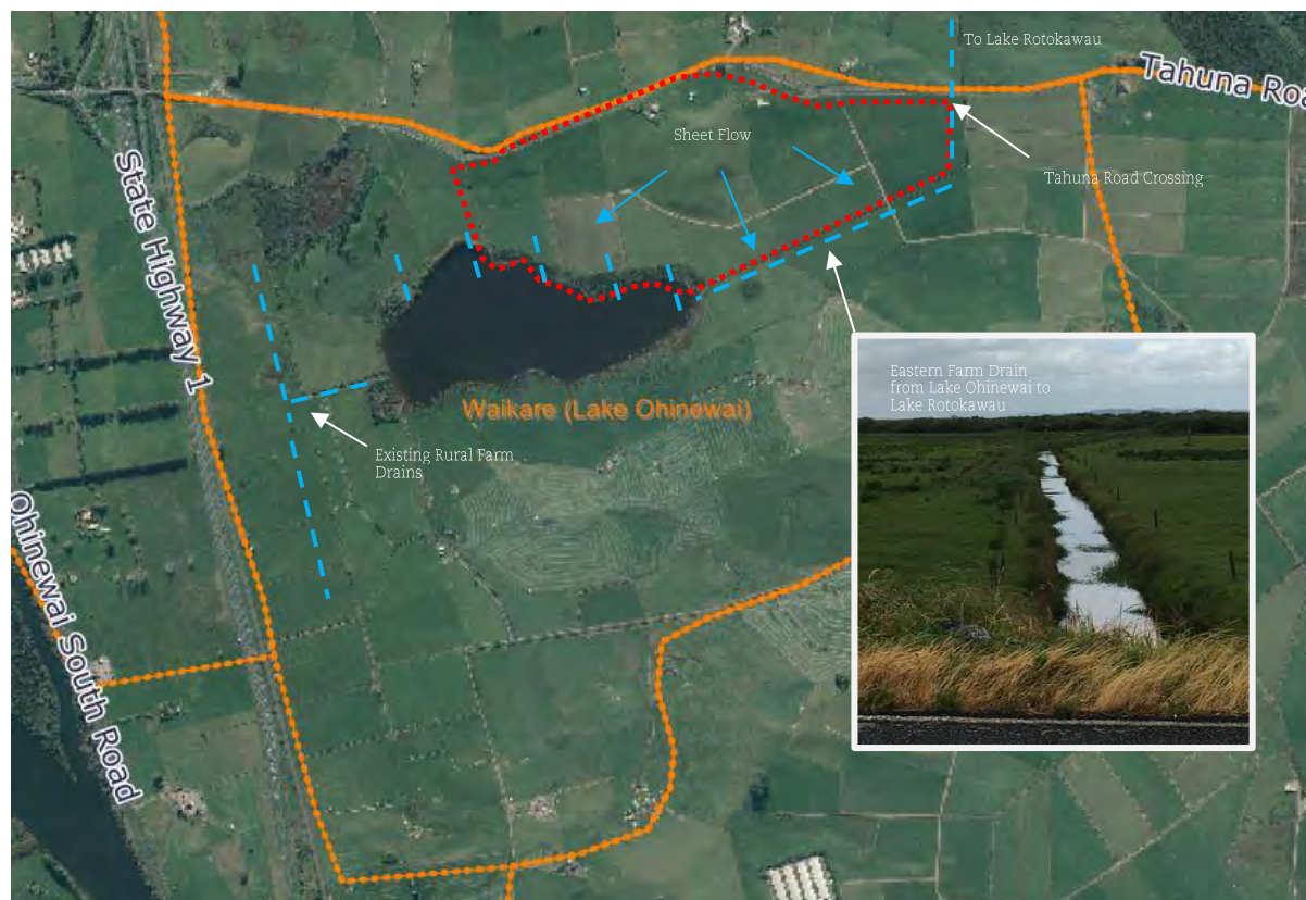
Figure 4: Waikere (Lake Ohinewai) Drainage District & Site Drainage Layout
