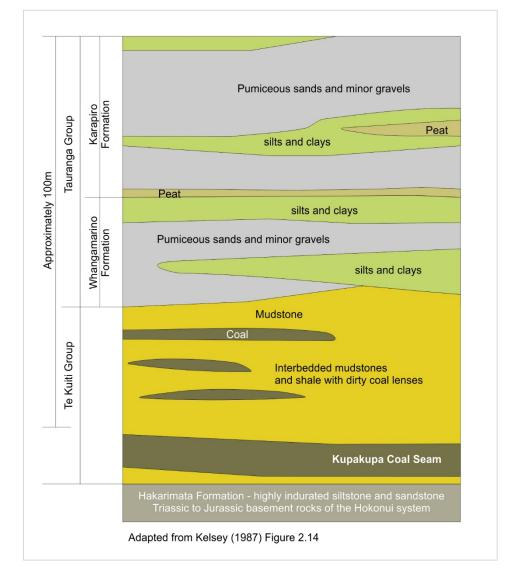
FIGURE 7 – SCHEMATIC ENGINEERING GEOLOGICAL PROFILE (KELSEY 1987)
