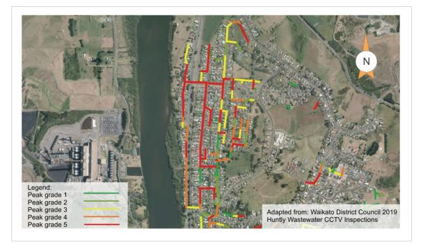
FIGURE 8 - WASTE WATER CCTV MONITORING
