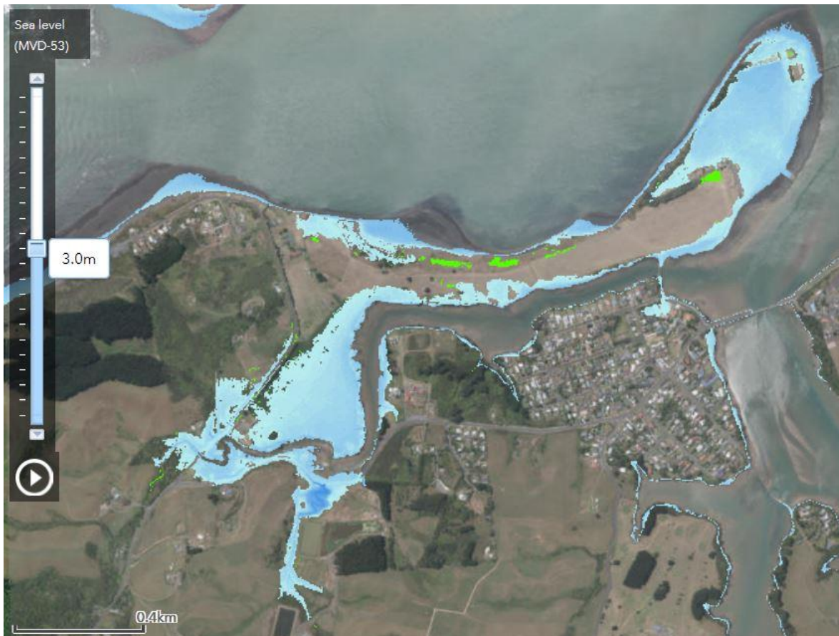
Figure 27: Illustration of the areas likely to be inundated (coloured) in a severe storm. Waikato Regional Council Coastal Inundation Tool http://coastalinundation.waikatoregion.govt.nz/ .
