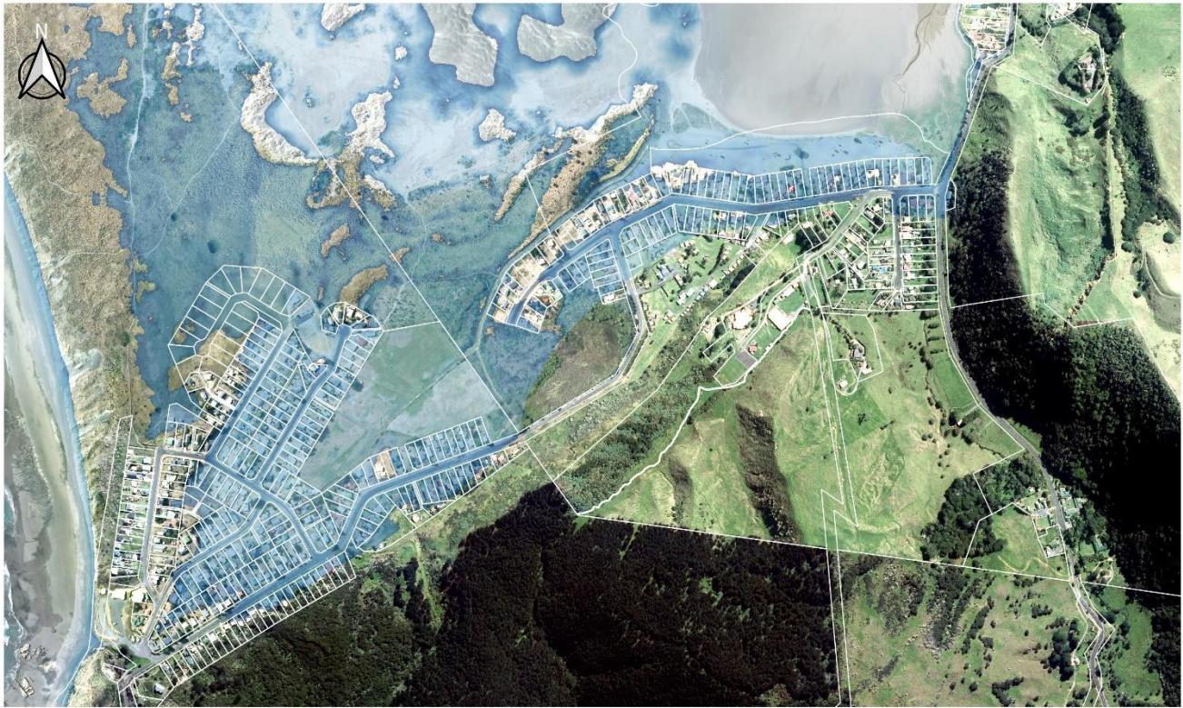
Waikato District Coastal Hazards - Coastal Inundation in extreme event with 1.0 m Sea Level Rise. Prepared by Focus Resource Management Group. © Waikato Regional Council 2018. Aerial Photography - Historic Aerial Photographs Data Sourced from http://retrolens.nz and licensed by LINZ CC-BY 3.0. Waikato - West Coast and Hauraki Plains LIDAR 1m DEM (2015) source from Waikato Regional Council licenced by Creative Commons Attribution 4.0 International.
