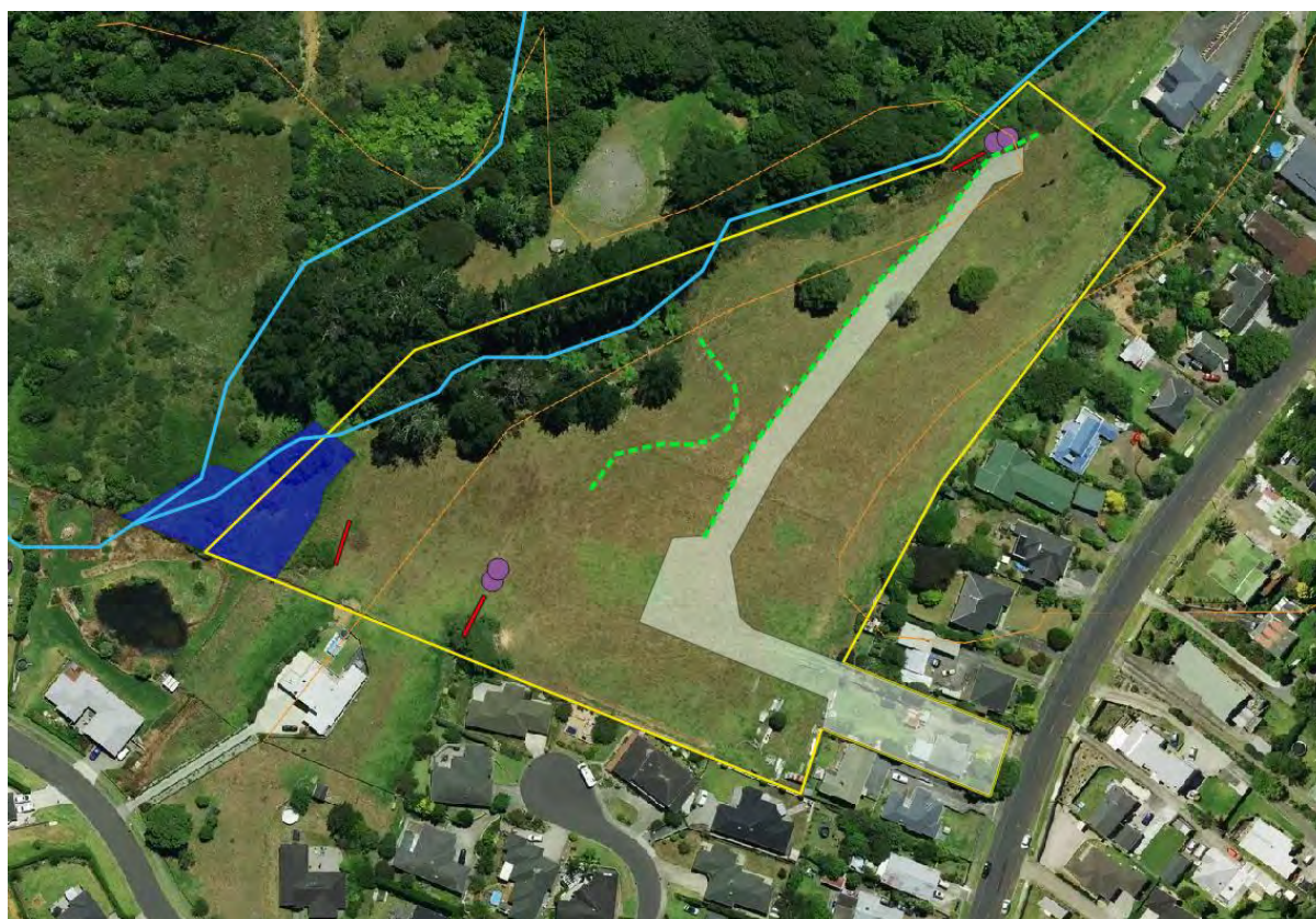
Figure 8: The proposed stormwater spreaders (red), stormwater tanks (purple), earthworks (white), and retaining walls (green), site contours (orange), overland flow paths (blue), pond (light blue) and wetland (dark blue).
