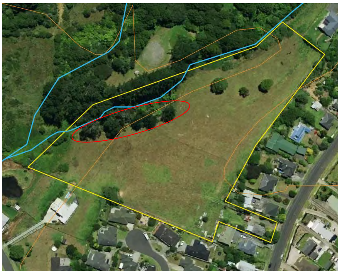
Figure 1: Map of the project site (site boundary in yellow) with overland flow paths (blue), contours (orange) and the indicative area of vegetation removal (red).
