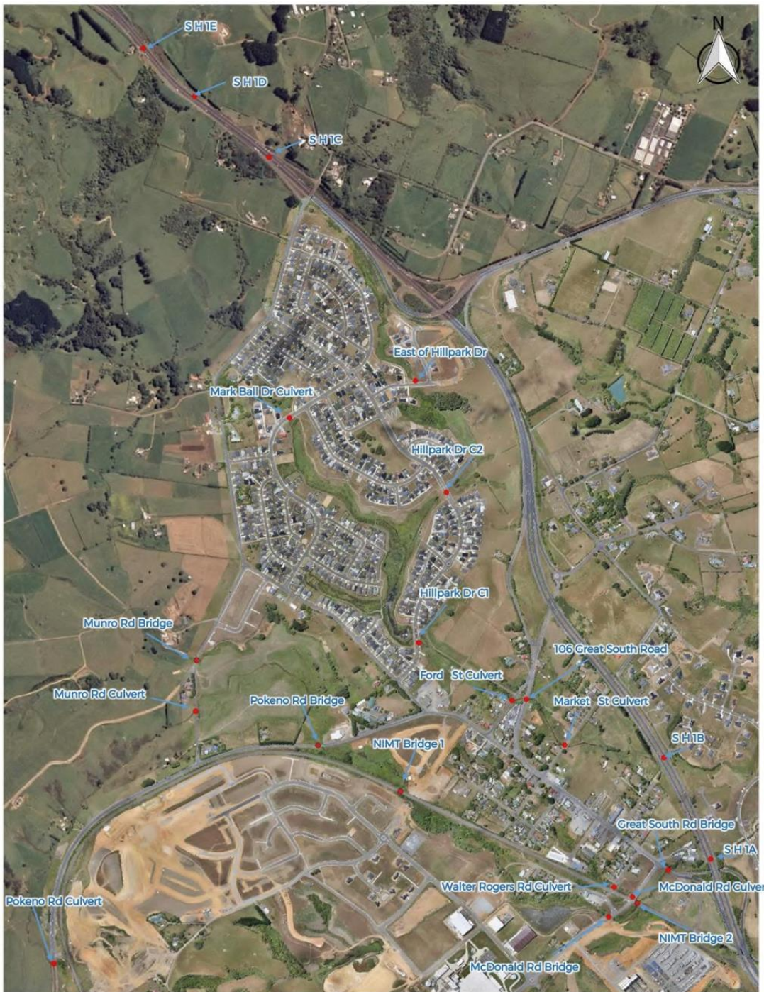
Figure 8-3: Bridge and culvert locations
