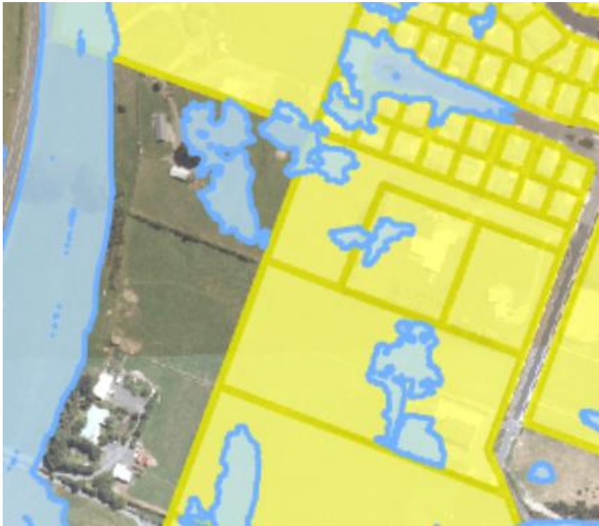
Figure 2: Te Miro flood and stormwater extents
