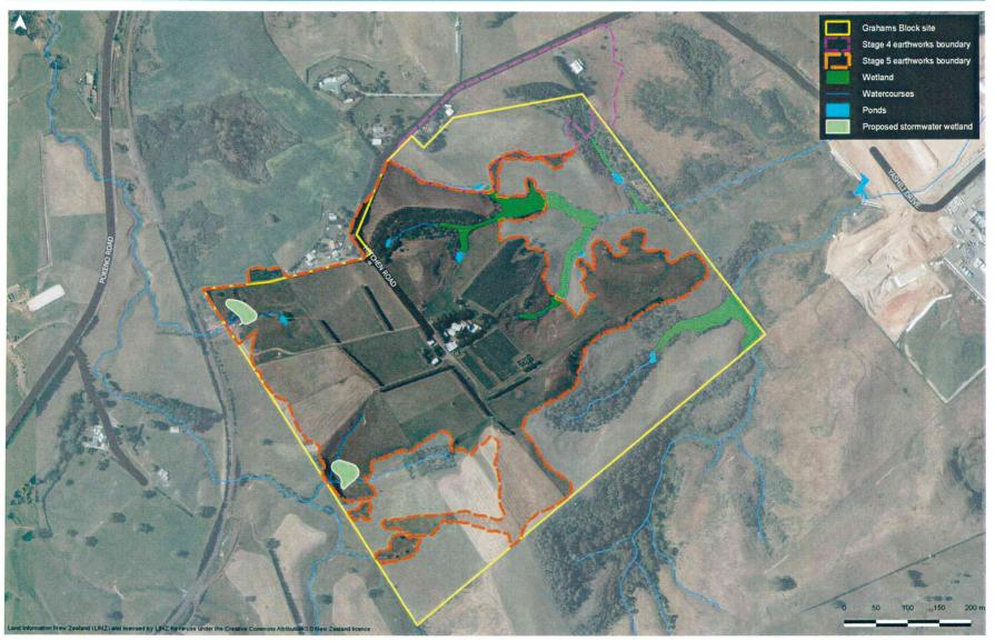
Figure 1: Stage 4 and 5 earthworks boundaries within the Graham Block site.
