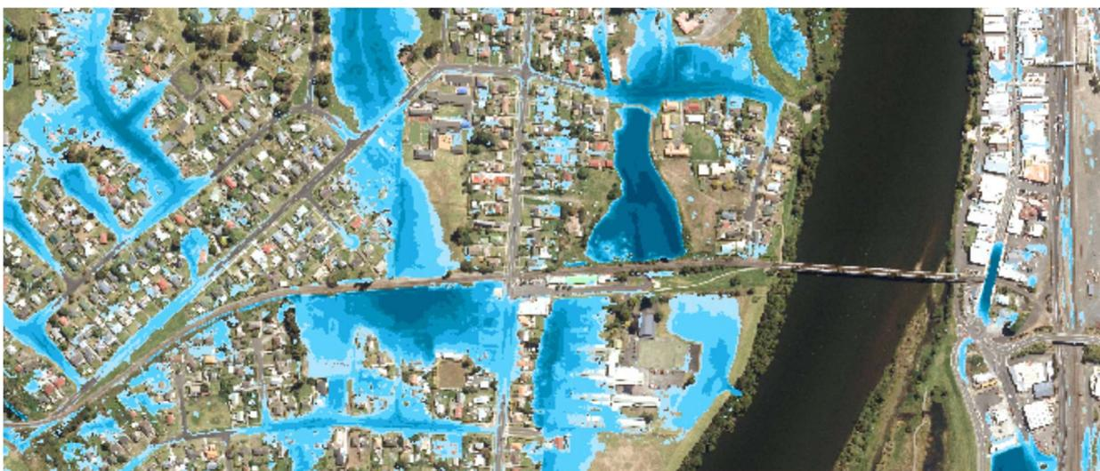
Figure 2: Blockage Scenario 1 – Shows increased flooding by the 100% blockage scenario. This shows an increase in flood levels but not significantly increasing the flood footprint. This blockage scenario is unlikely to occur as large culverts are less likely to completely block. As expected, there is no difference in areas that are not constrained by culverts. Result: Not considered a critical factor.
