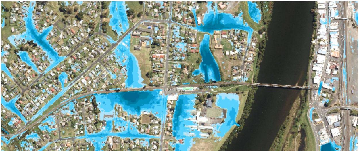
*Figure 4: CN Increased Scenario: Shows slight increase from base model (small isolated flooding areas not cleaned). Result: Not a critical factor in the flood model as very similar to base model.*
