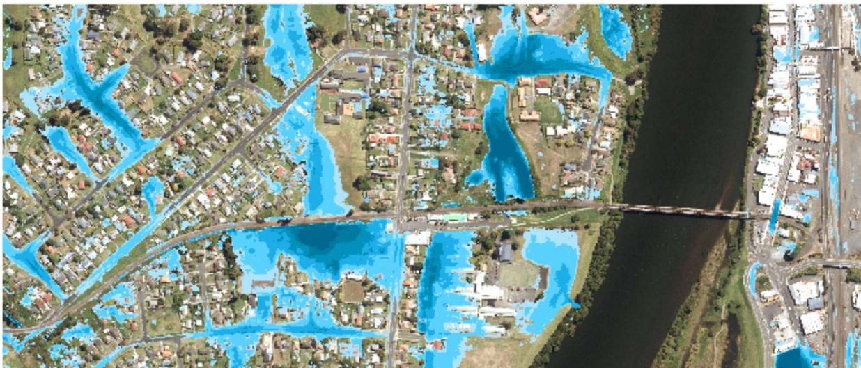
Figure 5: Increased Climate Change Scenario (RCP8.5): Shows slight increase from base model (small isolated flooding areas not cleaned). Very similar to the CN increase scenario. Result: Not a critical factor in the flood model as very similar to base model.
