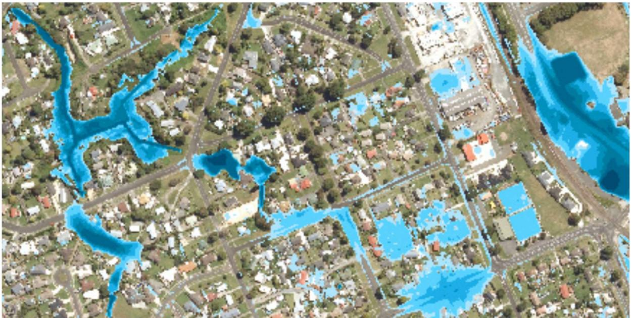
Figure 4: CN Increased Scenario: Shows slight increase from base model (small isolated flooding areas not cleaned). Result: Not a critical factor in the flood model as very similar to base model.
