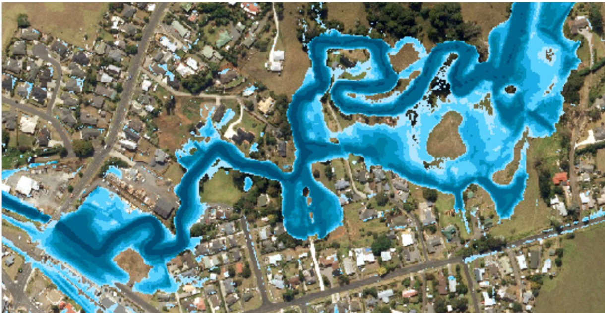
Figure 4: CN Increased Scenario: Shows slight increase from base model (small isolated flooding areas not cleaned). Result: Not a critical factor in the flood model as very similar to base model.
