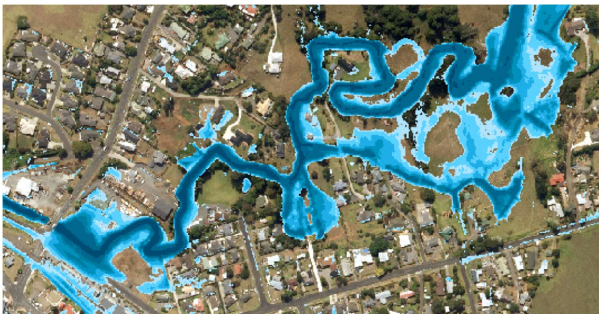
Figure 2: Blockage Scenario 1 – Shows increased flooding by the 100% blockage scenario. This shows an increase in flood levels but not significantly increasing the flood footprint. This blockage scenario is unlikely to occur as large culverts are less likely to completely block. As expected there is no difference in areas that are not constrained by culverts. Result: Not considered a critical factor.
