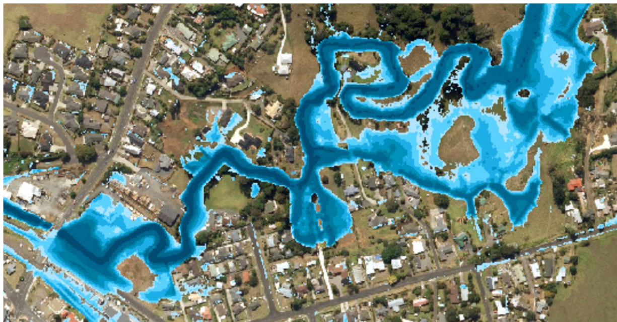
Figure 5: Increased Climate Change Scenario (RCP8.5): Shows slight increase from base model (small isolated flooding areas not cleaned). Very similar to the CN increase scenario. Result: Not a critical factor in the flood model as very similar to base model.
