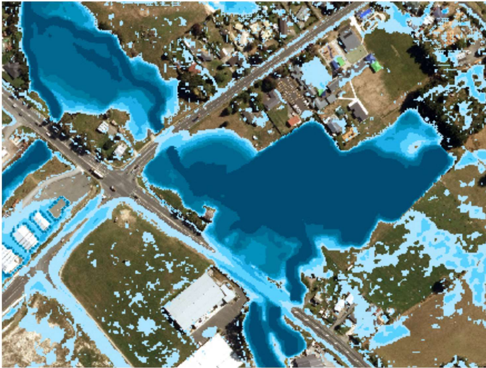
Figure 2: Blockage Scenario 1 – Shows increased flooding from 100% blockage scenario. Critical in areas upstream from large culverts but unlikely to occur as these large culverts are less likely to completely block. No difference in areas that are not constrained by culverts.
